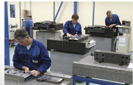
SiC Air Bearing Component assembly
