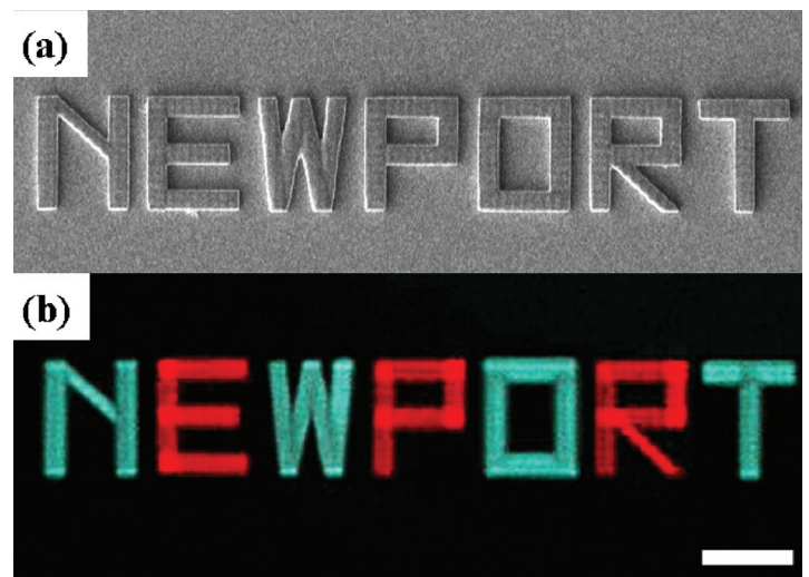
Figure 7 - SEM (a) and confocal microscopy (b) images of the word NEWPORT fabricated by TPP. The red and blue letters in (b) correspond to resins doped with Rhodamine B and Coumarin 334 respectively. The scale bar is 20 \mu\text{m} .
